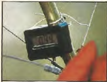
Fig.1. Calibration of the altimeter depends on setting the reference voltage supplied to the d.v.m. chip via the 100k \Omega calibration control. This derives from the voltage applied across the pressure transducer bridge thus ensuring perfect temperature tracking. The original instrument was calibrated against a certified aneroid barometric altimeter taken to 5500ft from airfield level. Readings related better than one per cent at all intermediate levels following calibration.
